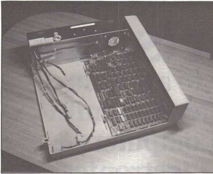
HF-148-41 cabinet with both the supply and CPU board installed.
