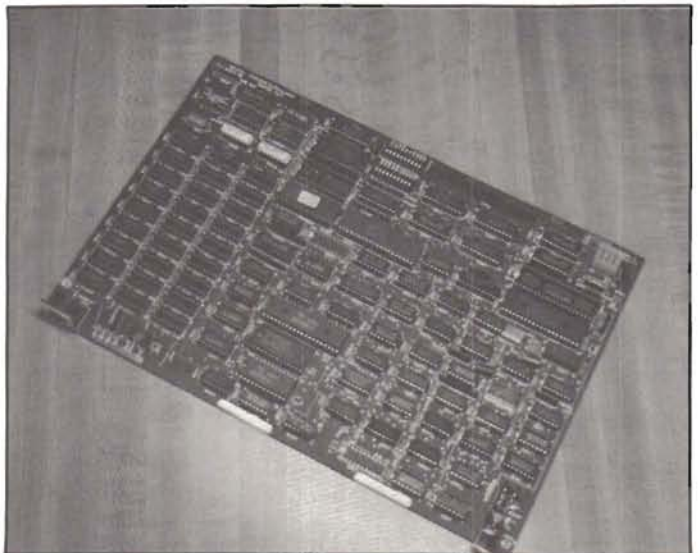
Pre-assembled CPU board ready for installation.
