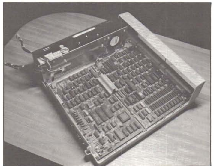
Only the drive(s) need to be installed to complete the assembly of the HF-148. Extra memory and/or the 8087 should be installed before the drive(s).
