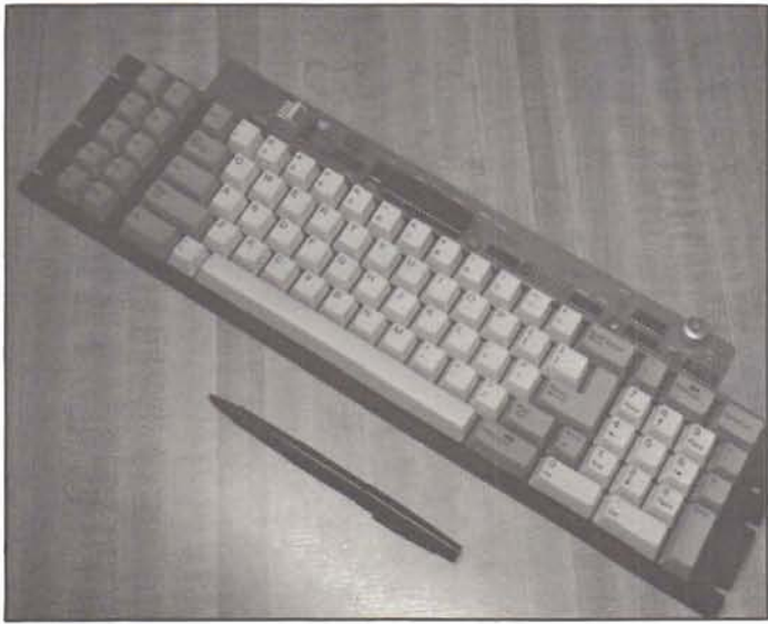
Assembled keyboard ready for installation in keyboard cabinet shell.
