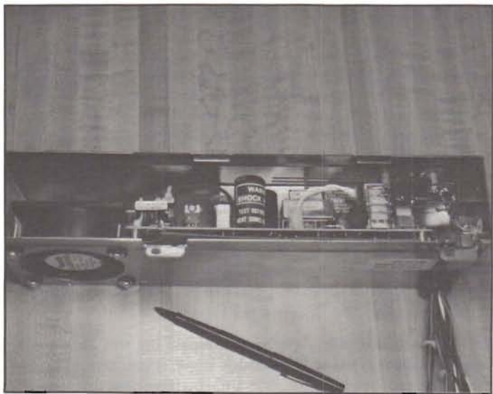
Pre-assembled supply ready to be installed in HF-148-41 cabinet.
