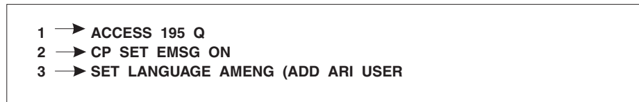
Figure 87. PROFILE EXEC Entries for a User Machine
