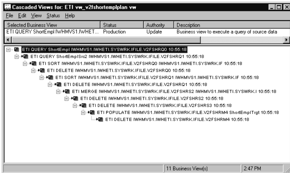
Figure 15. Sequence of generated business views. The selected business view is the one to start manually.
