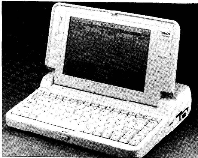
Photo 61. Tandy's upgrade to their popular 1100FD, the 1110HD, adds a 20MB hard drive without adding undue weight or increasing its size.
