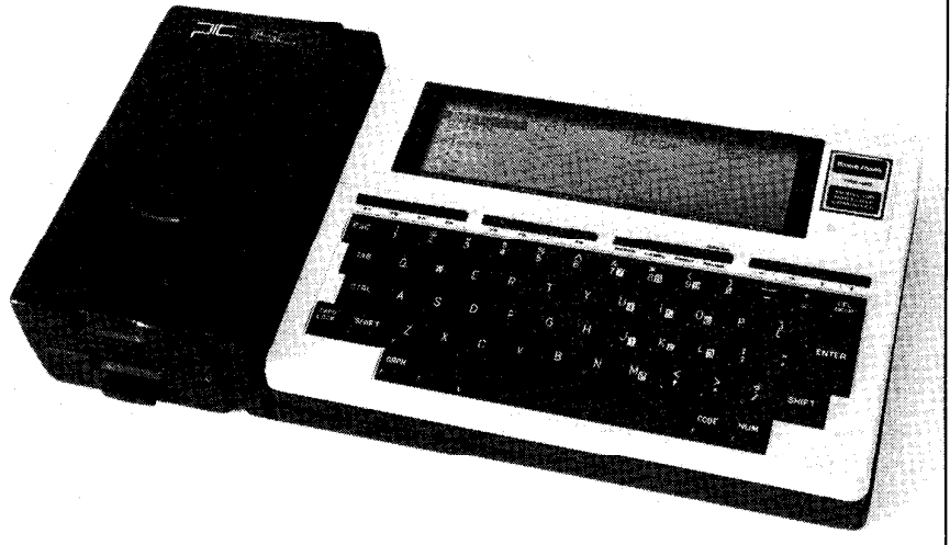
The PIC Disc attaches to the bottom of the 100 with screws and velcro strips, forming a single conveniently portable package.
