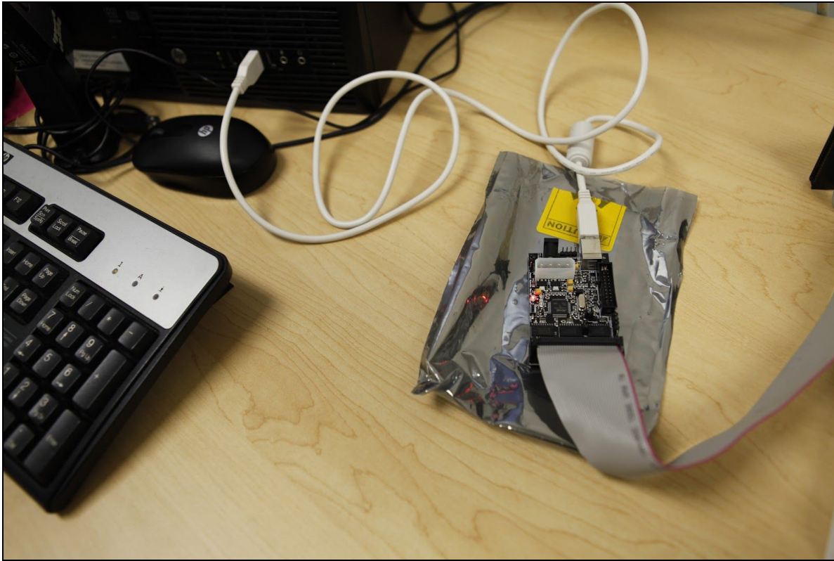
Figure 5: Once the drive is connected to the KryoFlux board via the data cable, connect the board to the computer using the USB cable.
